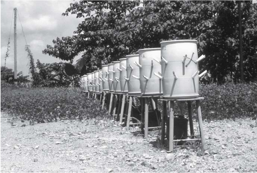
Fig. 2.12. Drums used for the kinetic testing of sulfidic mine wastes at the Misima Island gold mine, Papua New Guinea. The tubes enable meteoric water and atmospheric gases to interact with the waste, and leachate can be collected from the drum base
