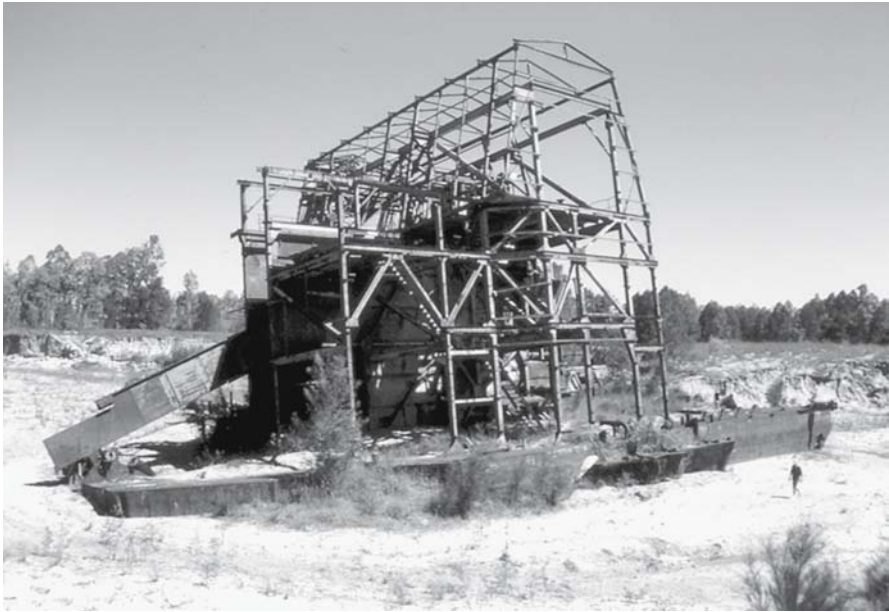
Fig. 1.7. Abandoned tin dredge in the dry stream bed of Nettle Creek, Innot Hot Springs, Australia. The bucket dredge was used in the 20th century to extract alluvial cassiterite. During mining, the dredge caused a massive increase in suspended sediment loads and the deterioration of stream water quality. Consequently, the Mining Act Amendment Act 1948 was introduced which is one of the first pieces of Australian legislation specifically concerned with environmental protection. The act required operators to construct settling ponds for turbid mine waters
