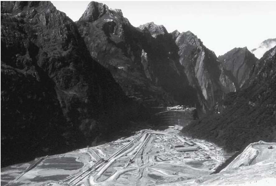
Fig. 1.9. The Ertzberg open pit, Irian Jaya, Indonesia. The Grasberg-Ertzberg mine – located at about 4 000 m among the jagged alpine peaks of the Jayawijaya mountain range – is one of the world's largest mining operations. Approximately 0.24 Mt of copper ore are mined every day, and 0.2 Mt of tailings are dumped into the Ajkwa River system every day, causing increased sedimentation on the coastal floodplains
