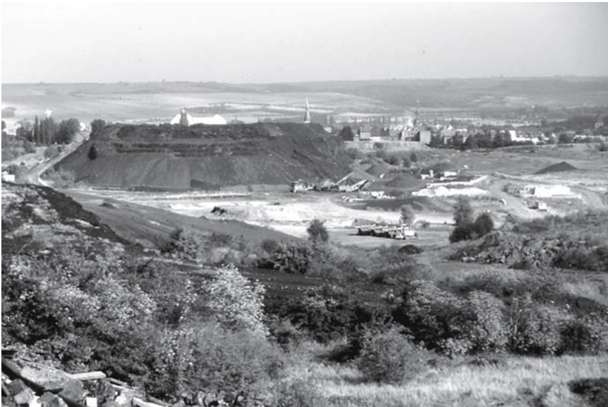
Fig. 1.8. Abandoned slag and waste heaps of copper ores, Eisleben, Germany. Mining in the area occurred for over 800 years, resulting in over 2 000 individual waste heaps, 1 000 km of underground workings and 56 million cubic meters of mine voids. Under the East German communist regime, the extraction of metals from very low grade, uneconomic copper ores was pursued, and large volumes of fly ashes, tailings, and smelting slags were generated. The unconstrained release of wastes into the local environment, especially of atmospheric emissions from smelting works, has caused widespread contamination of streams and lakes with metals and metalloids
