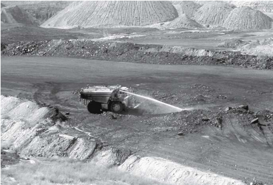
Fig. 2.6. Water spraying of spontaneous combustion at the Blair Attoll coal mine, Australia (Photo courtesy of P. Crosdale)
