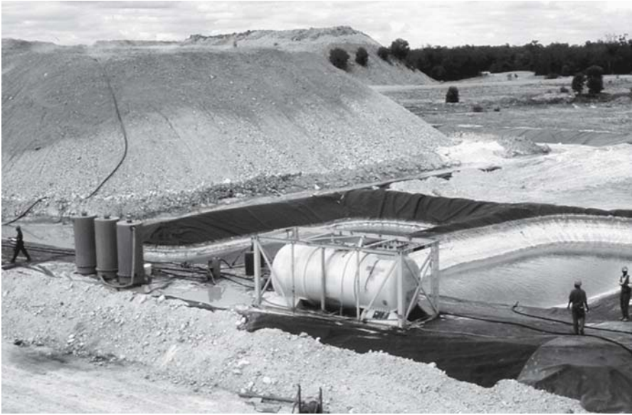
Fig. 5.2. Cyanide heap leach pile and plastic lined collection ponds, Wirrallee gold mine, Australia
