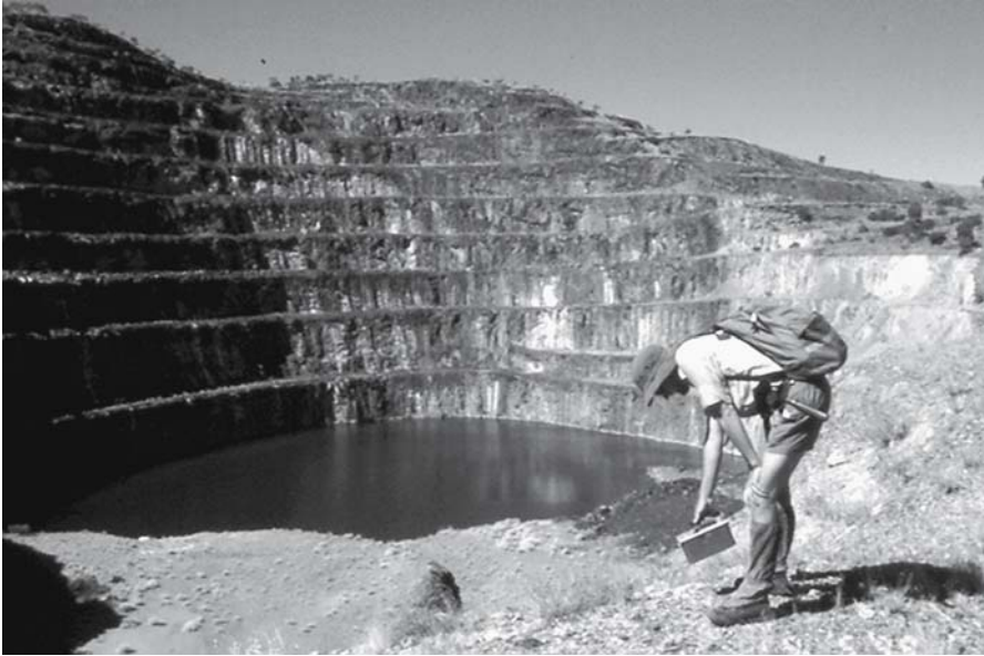
Fig. 6.1. Open pit of the Mary Kathleen uranium mine, Australia. Elevated gamma-ray readings in the open pit correspond to exposed ore lenses, the former haul road, and abandoned ore stockpiles (up to 16 mSv per year). Wallrock oxidation of reactive sulfides produces acidic solutions, yet buffering reactions prevent low pH conditions from developing. The open pit lake contains saline surface waters at a pH of 6.11 (salinity 0.15‰; elevated Ca, SO 4 , Cu, Fe, Mn, Ni, U and Zn values)
