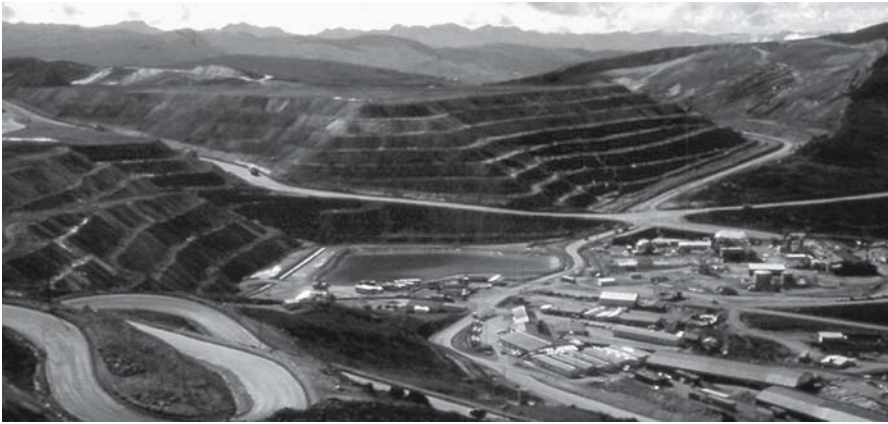
Fig. 5.3. Large heap leach piles at the Yanacocha gold mine, Peru. The siliceous gold ore is so porous that it can be heap leached without crushing. (Photo courtesy of P. Williams)
