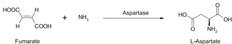
Fig. 5 Enzymatic reaction catalyzed by aspartase from E. coli
