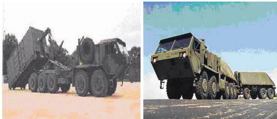
Fig. 1. On left: Modular Vehicle with ISO Module and Integral Load Handling System 7 . On right: Modular Vehicle with Integral Load Handling System and Modular Trailer both with Flat Rack Modules 8 .
