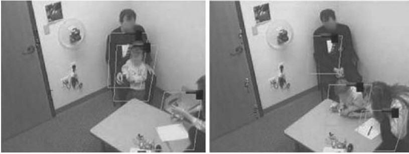
Fig. 3. Two tracking images from the left camera of a calibrated stereo cameras rig. Individuals are tracked as they move throughout one of our clinical evaluation rooms during an interview session.
