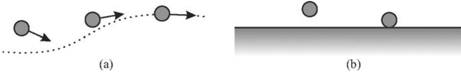
Fig. 3. (a) Guidance virtual fixtures assist in guiding the robot along desired paths. (b) Forbidden-region virtual fixtures help keep the robot out of forbidden regions.
