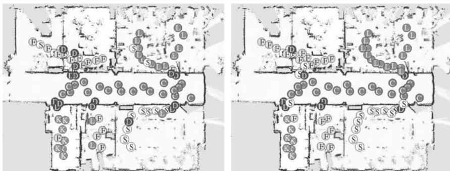
Fig. 10. The left image depicts a typical classification result for a test set obtained using only the output of the sequence of classifiers. The right image shows the resulting classification in case a HMM is additionally applied to filter the output of the sequential classifier.
