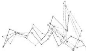
Fig. 6. Subjective localization of the robot using the camera. Dotted line is ARE's trajectory on training data, solid line is predicted location using MCL on test data.
