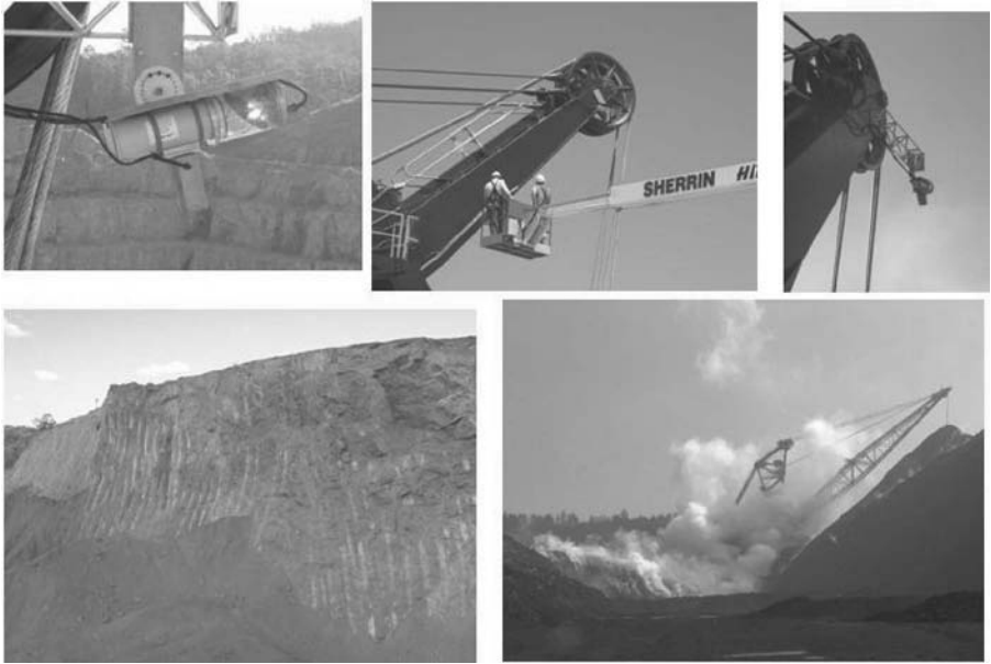
Fig. 7. Millimetre Wave radar installed in a rope shovel
