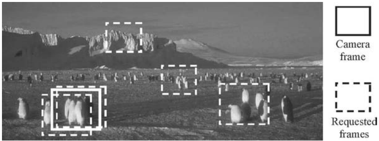
Fig. 4. Panoramic image and user or machine-requested “activity frames”.
