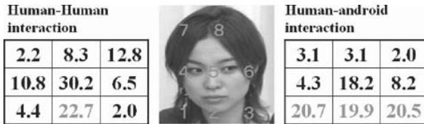
Fig. 10. Comparison between human-human interaction and human-android interaction. The gazing directions are represented by 9 areas with the numbers representing percentages.
