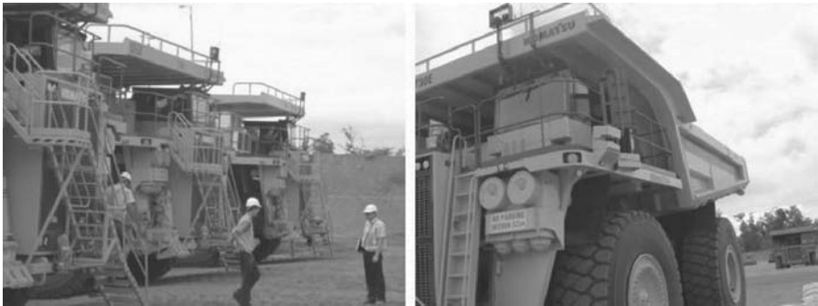
Fig. 11. Truck fleet and a truck retrofitted with a laser based tracking system
