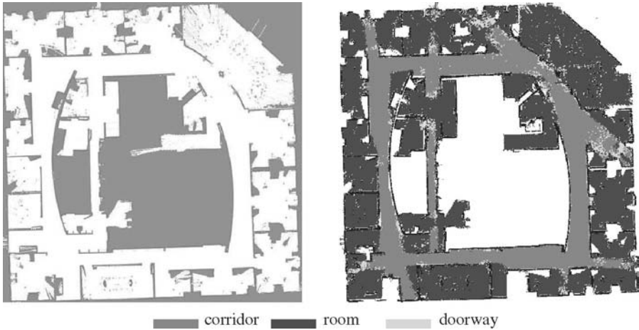
Fig. 8. The left map depicts the occupancy grid map of the Intel Research Lab and the right image depicts the classification results obtained by applying the classifier learned from the environment depicted in Figure 1 to this environment. The fact that 86.0% of all places could be correctly classified illustrates that the resulting classifiers can be applied to so far unknown environments.
