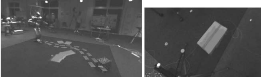
Fig. 9. Environment reconstructions overlaid onto the world. (a) Occupancy grid generated from image-based reconstruction using the robot’s camera. (b) planar projection of an obstacle recovered from range data.
