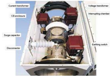
Fig. 8. Main assembly of GCB.
