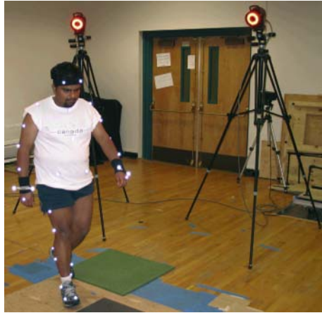
Figure 1: Highly reflective optical markers placed on a motion capture subject.
