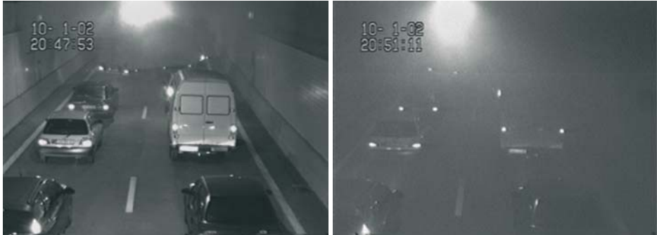
Figure 4: One of the tests of Study 2. (Pictures taken 1'31" and 4'49" after the stop of the truck in front; test participants don't leave.).
