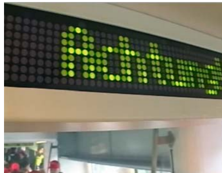
Figure 2: Illuminated passenger information display underneath the ceiling situated in the exit area of each door
