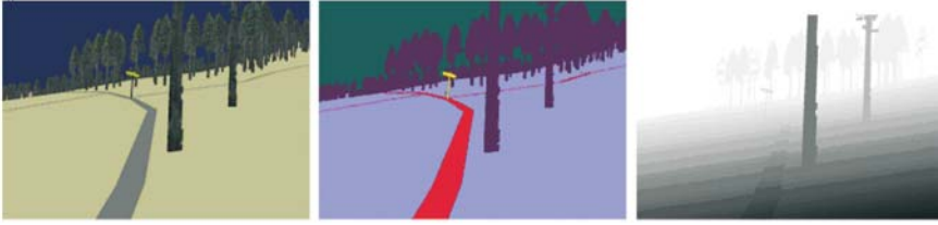
Figure 6: The visibility analyzer module calculates what can be seen by each agent in the simulation. Using positional data generated by the physical simulation, the module uses 3D rendering techniques to render false colour images and depth maps of the agent’s field of view. These images are analyzed and information about what is seen is broadcast back to the event stream.
