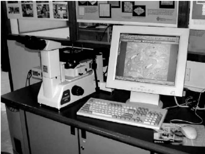
**Figure 2.** Nikon Epiphot 200 inverted light microscope on line with a computer to monitor the bone surface topology
