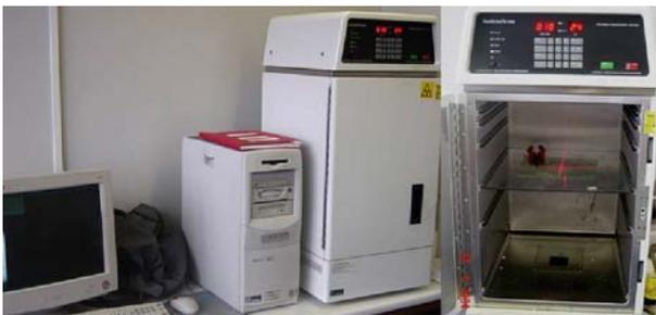
**Figure 1.** Faxitron MX-20 digital radiography system
