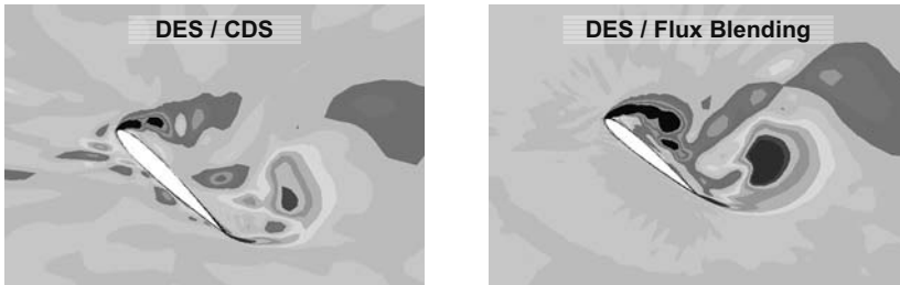
Figure 5 Distribution of the predicted instantaneous vorticity contours \omega_z at mid span ( z/c = 0.5 ) in response to the applied approximation of advective fluxes. Results refer to the SA model.
