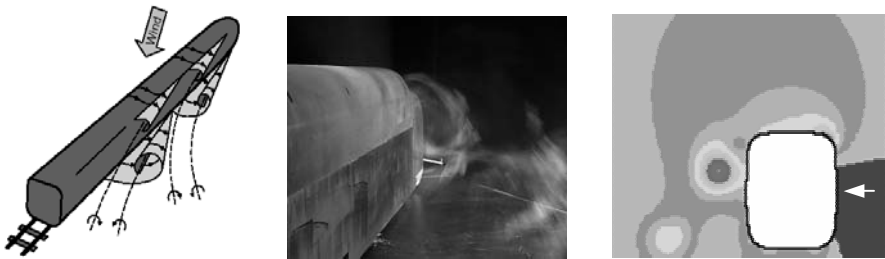
Figure 2 Illustration of the leeward vortices of a train exposed to cross winds (left); Flow visualisation from a wind-tunnel experiment (middle); Predicted pressure contours half a car downstream of the nose for 30° yawing (right).
