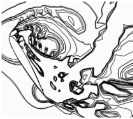
a) Roll-up and separation of leading edge vortex (Maximum C_l )
