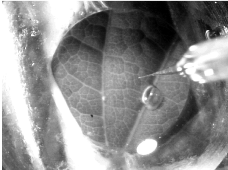
Fig. 20.2. Microcapillary made of borosilicate is used as an electrode in order to impale plant cells and detect V_m
