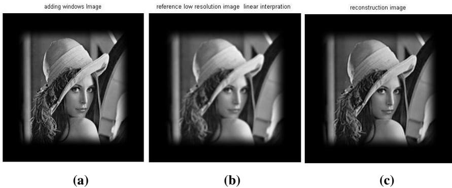
Fig. 2. (a) The original high resolution lena image added Tukey window. (b)the linear interpolation image. (c)the POCS super-resolution reconstruction image based on the registration algorithm excluded aliased frequency domain.
