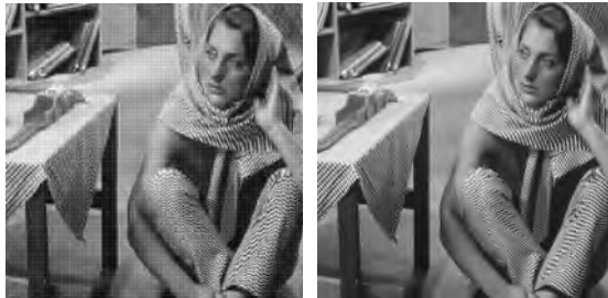
Fig. 4. Comparison at 0.2 bpp. Left: contourlet EBSSM; Right: wavelet SPECK.
