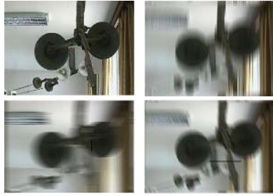
Fig. 1. Different camera motions lead to different motion blurs. Here, in top right corner and bottom left corner, the unblurred still image (top left corner) is blurred by linear vertical and horizontal motions, respectively. In bottom right corner, the image is blurred due to motion blur with an angle.
