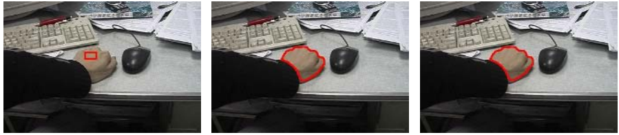
(a) the original image and the initial curve (b) the result of the original model after 30 iterations (c) the result of the improved model after 30 iterations
