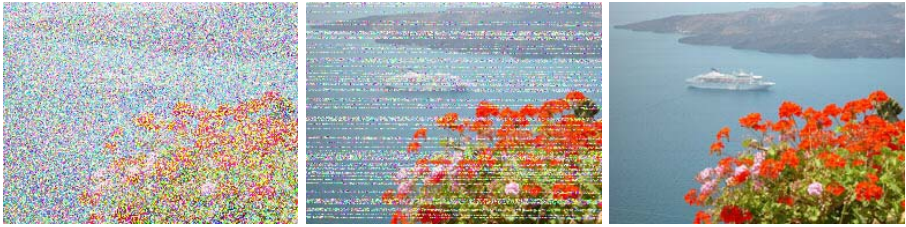
Fig. 3. A sample image corrupted by the additive white Gaussian noise channel of the signal-to-noise rate Eb/No = 1.8 dB (left). Belief propagation (middle). Cooperative optimization (right).
