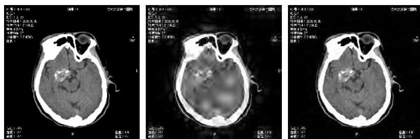
Fig. 2. The comparison of compression results with different IWT schemes for the CT1 image at 0.25bpp. The original image (left); the reconstructed image without the OSS scheme (medium); the reconstructed image with the OSS scheme (right).
