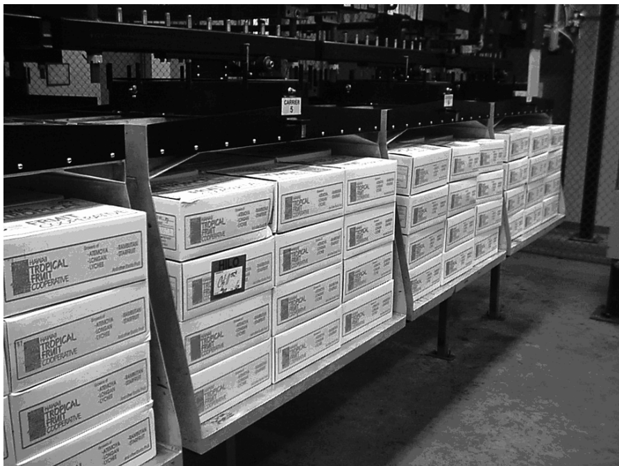
Fig. 21.1 Boxes of papayas two boxes deep on a conveyor system to be irradiated by X-rays for phytosanitary control of tephritid fruit flies in Hawaii before export
