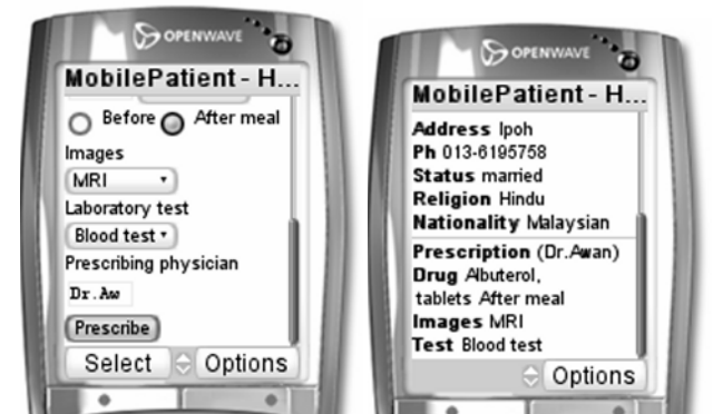
Fig. 4 Openwave Phone Simulator display of a) the form to add prescription data, b) the updated patient details
