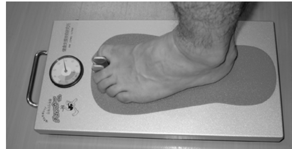
Fig.1 The measurement device of toe-gap force
