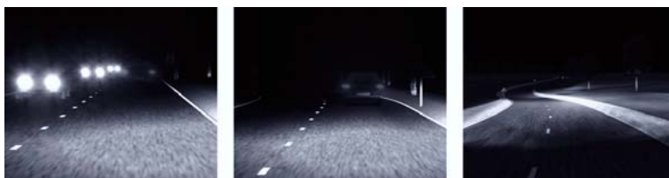
Fig. 5.52 Renault's driving simulator: simulation of glare from oncoming traffic (left), tail lights (centre), and headlamps (right) during a simulated night drive (Source: OKTAL SA, France)
