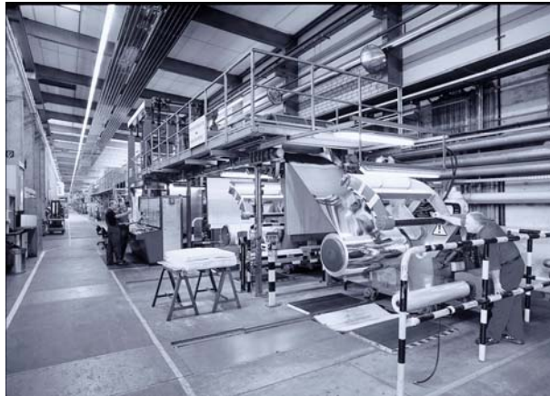
Fig. 3.123 Industrial continuous coil anodising (Alanod 2005)
