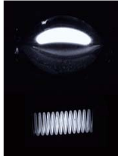
Fig. 3.102 comparison of arc of a gas discharge light source (above) with the filament of a halogen bulb (below)
