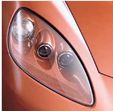
Fig. 3.42 Concealed headlamp using body colour bezel (source: Visteon)
