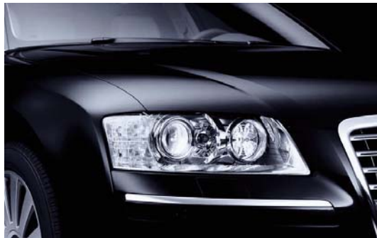
Fig. 3.59 Separate day time running light (right) with white LEDs (source: Audi)
