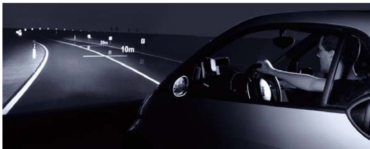
Fig. 5.53 Hella's night drive simulator 'Light Driver' in the L-LAB
