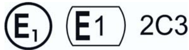
Fig. 3.98 E-sign in its conventional form (left) and as allowed if the space is limited (right, from a bulb together with the certification number)
