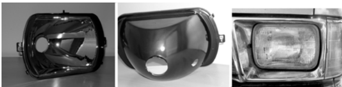
Fig. 3.114 Old style sheet metal reflector in parabola shape (source: Visteon) and SAE glass sealed beam
