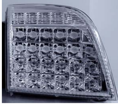
Fig. 3.19 First Visteon LED Headlamp demonstration prototype from 2002 (source: Visteon)
