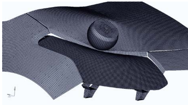
Fig. 3.32 simulation of child head impact of front end of the car (source: Visteon)
