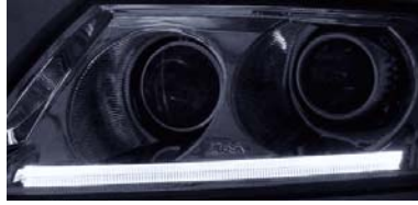
Fig. 3.71 Example of a light guide as a front position light. The light guide highlights the bottom edge of the headlamp. It creates a stylistic feature that totally changes the appearance of the headlamp. Two white LEDs with Lambertian characteristics feed the light guide (source: Visteon)
