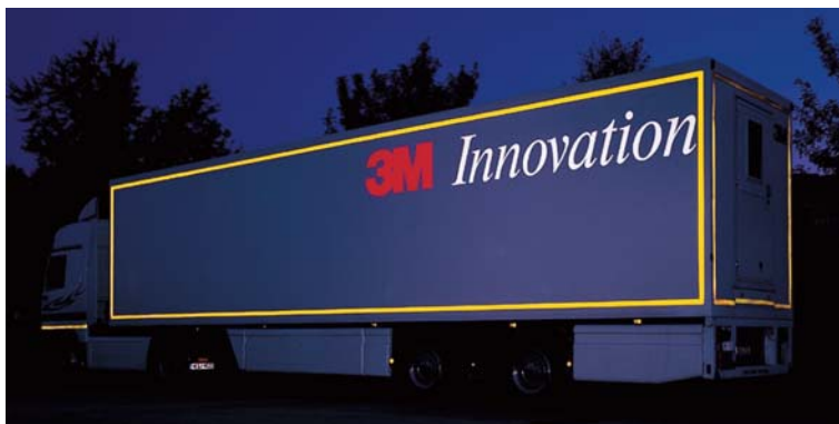
Fig. 2.48 Passive contour marking using reflective foil (source: 3M)
