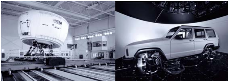
Fig. 5.51 NADS - High-end driving simulator with 360°-projection dome and hexapod on top of a 2D linear motion system (left) and high frequency actuators driving the vehicle chassis inside the dome (right). (Source: NADS, University of Iowa)
