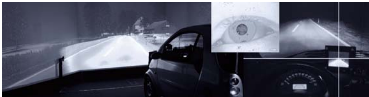
Fig. 5.55 L-LAB-set-up of the virtual night drive-simulator (left) and examination of driver behaviour using eye-tracking (right)
