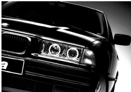
Fig. 3.75 Example of a position lamp with light guide (source: Hella)
