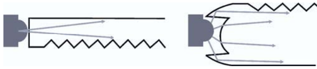
Fig. 3.62 Example of light coupling from LEDs
