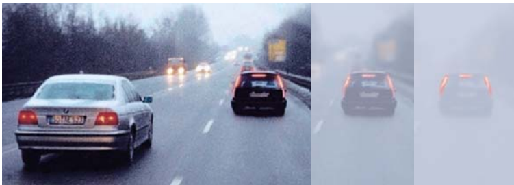
Fig. 2.50 Contoured signal lights are easier to pick up in low contrast conditions
