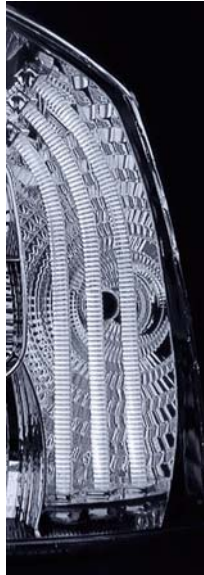
Fig. 3.72 This example shows light guides that highlight the outside edge of the rear lamp and function as a position light. Six LEDs with narrow radiation pattern feed three light guides from both ends (source: Visteon)
