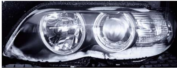
Fig. 3.35 Water condensation on the outer lens of a headlamp
