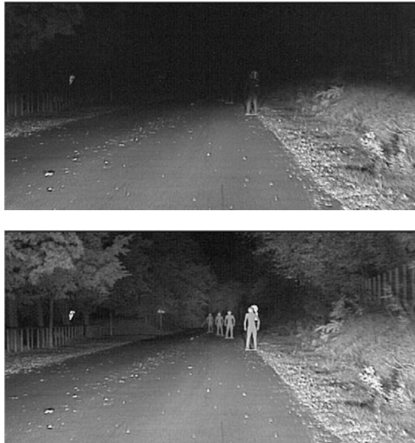
Fig. 3.57 Comparison without (top) and with night view assist (bottom) (source: DaimlerChrysler)
