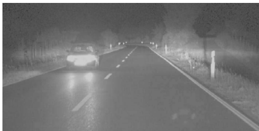
Fig. 3.53 : Night vision image from DaimlerChrysler experimental laser/CCD system (source: DaimlerChrysler)
