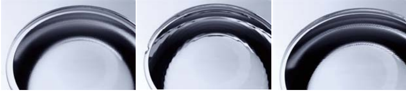
Fig. 3.127 Textured lens surfaces; frosting (left), modulation, microstructure (right)
