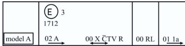
Fig. 3.51 Example of AFS approval markings
