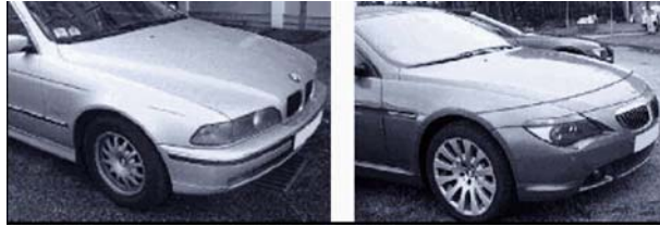
Fig. 3.134 Difference in front-end styling – older sharp design with ordinary shape of headlamp design (left) and new smooth styling of front-end with shaped headlamps (right)
