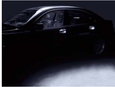
Fig.5.23 Entrance/Exit light activated by remote door opener (Source: Hella)
