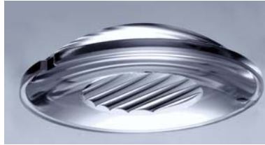
Fig. 3.129 Wave structures on the planar side of an aspheric lens
