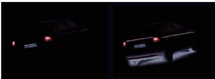
Fig. 2.49 Under floor lighting (right) accentuates the contour of the vehicle
