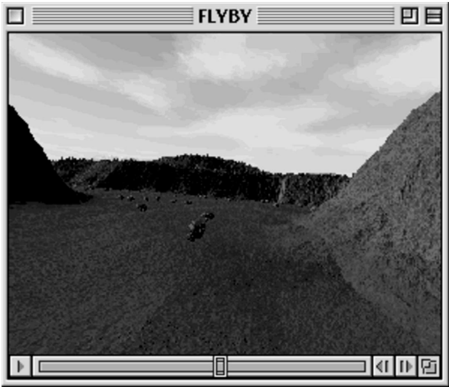
Fig. 4. Animation and changing representation. The change can be due to data or graphic manipulation. The fly-through of a mountain area in the south of France is represented here with two frames, and is an example of the last category. To create the animation the user can define a path in a map and set the distance between the locations in the landscape where the subsequent frames will be generated.
