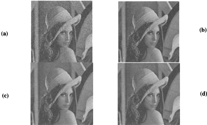
Fig. 8. Corrupted Lena image (a), and outputs of: median filter with 3x3 window (b), ten iterations of median filter (c), and proposed algorithm (d)
