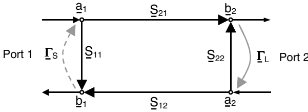
Fig. 3.8. Calculation of \underline{\Gamma}_{11} = \frac{b_1}{a_1} of a device characterised by its S-parameters and terminated by an output load with \underline{\Gamma}_L using Mason's rule
