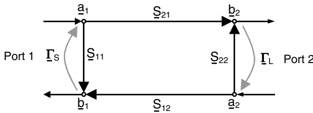
Fig. 4.4. Signal flow diagram of 2-port for calculation of transducer gain
