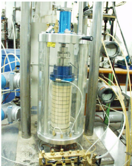
Fig. 18.23 Hollow cylindrical specimen undergoing consolidation (by G. Arangelovski)
