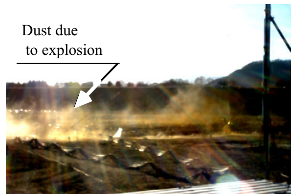
Fig. 18.14 Explosion to trigger liquefaction
