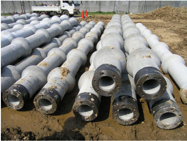
Fig. 13.31 Nodular piles prior to installation
