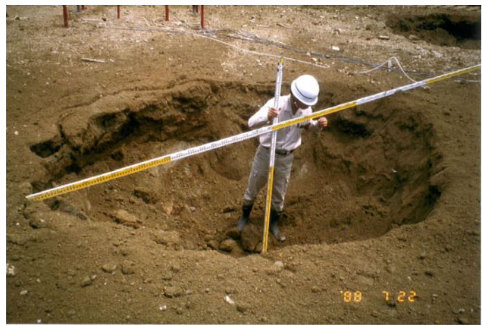
Fig. 26.68 Big hole made by impact energy of free fall (at Mizushima)
