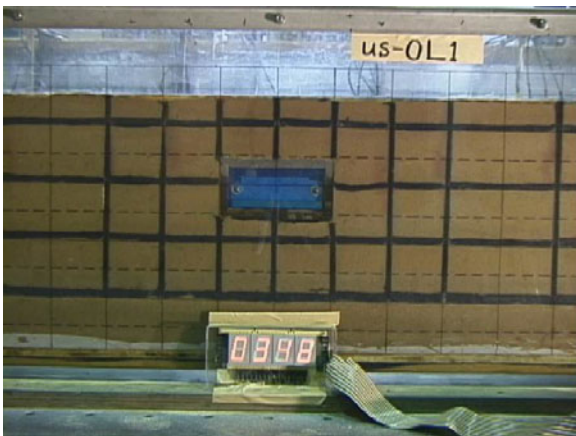
Fig. 26.38 Floating test on model without mitigation
