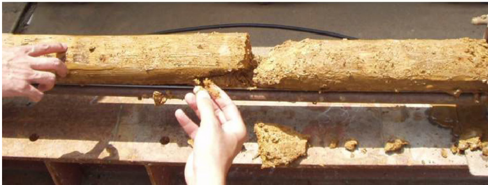
Fig. 10.58 Collected undisturbed soil sample by tube sampling method
