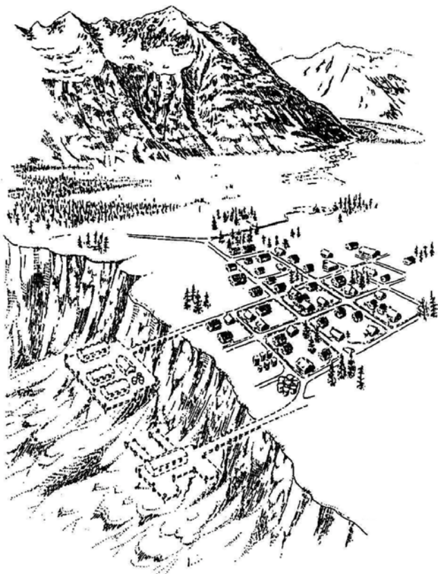
Fig. 15.52 Conceptual sketch of Valdez submarine landslide (Drawn by David Laneville; after Coulter and Migliaccio, 1966)
