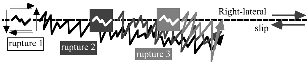
Fig. 16.20 Schematic illustration of preferred orientation of strong motion caused by strike-slip fault action
