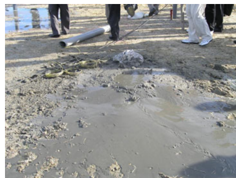
Fig. 26.142 Liquefaction caused by blasting
