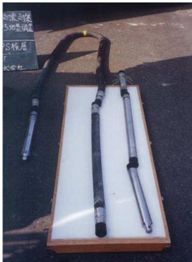
Fig. 8.6 Suspension survey equipment on site
