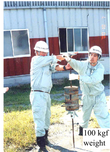
Fig. 8.32 Rotating Swedish weight sounding device (100 kgf=0.98 kN)
