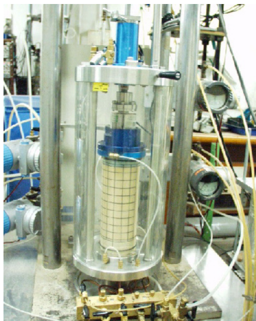
Fig. 18.23 Hollow cylindrical specimen undergoing consolidation (by G. Arangelovski)
