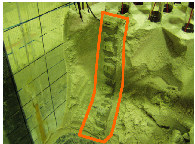
Fig. 24.56 Inclinometer upon excavation after liquefaction test (Photo by R. Motamed)
