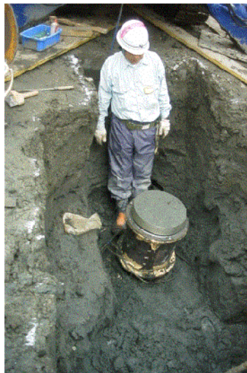
Fig. 10.60 Large block sampling of Yurakucho sand in Tokyo by Fujiwara et al. (2005)
