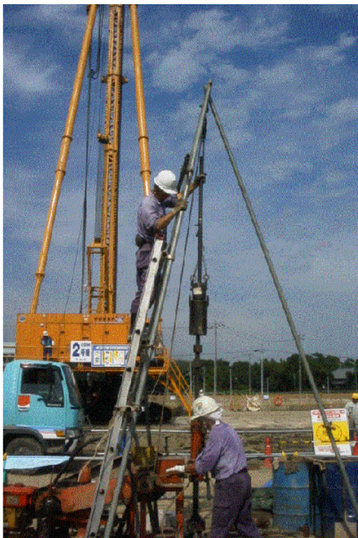
Fig. 1.38 Example of free-fall standard penetration equipment
