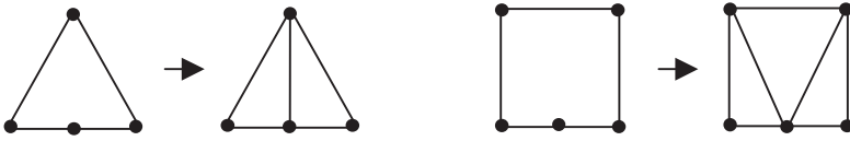
Fig. 2. Subdivision of elements with one saturated edge
