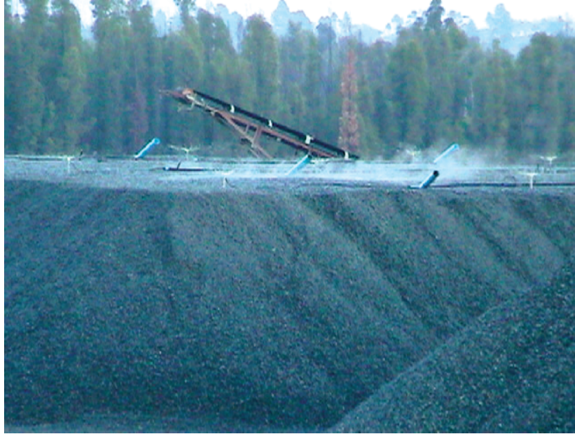
Fig. 5.7. Irrigation of the heap surface
