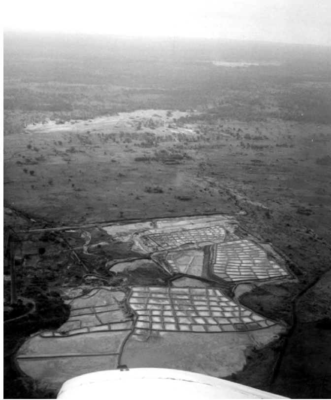
Fig. 2.1. Aerial view of the pyrite concentrate stockpile before the implementation of the bioleaching plant. In the background, devegetated areas downhill from the stockpile due to pyrite run-off
