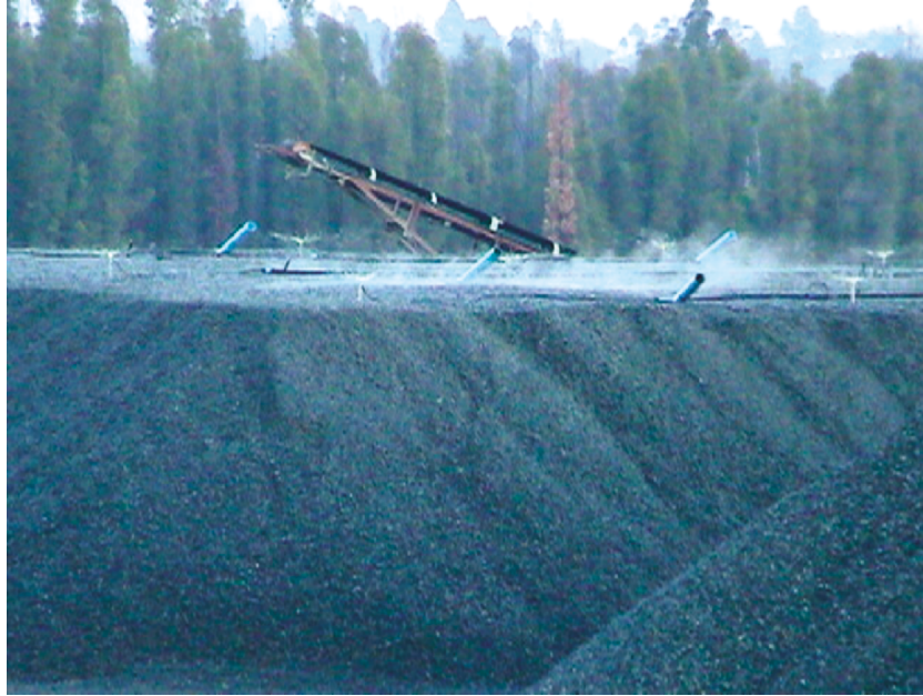
Fig. 5.7. Irrigation of the heap surface
