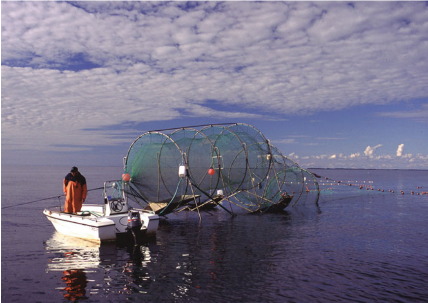
Fig. 6 Seal safe pontoon trap for salmon with doubled net walls. Photo: Pekka Salmi
