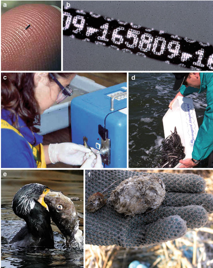
Fig. 2 Small individually or batch coded pieces of steel wire (coded wire tags) were used to mark fish. After release the proportion of fish eaten by cormorants can be estimated by counting the tags in regurgitated pellets by the use of a special metal detector. Photos a–c: Northwest Marine Technology Inc., d, f: Niels Jepsen, e: Per Huniche Jensen
