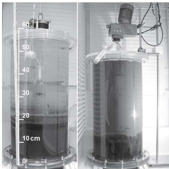
Fig. 6.27. “Water column simulator” with inserted DGT devices before start of the resuspension, and during resuspension of the anoxic layer. The inner diameter of this device is 29 cm and the used height is 59 cm
