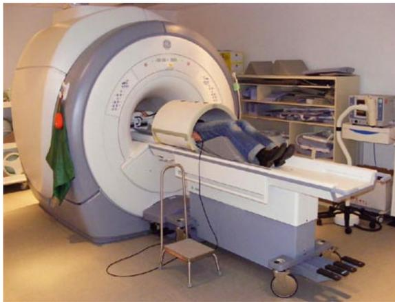
**Fig. 4.1.5.** Custom birdcage quadrature body transmit-receive coil for  $^3\text{He}$  at 1.5 T described in DE ZANCHE et al. (2008)
