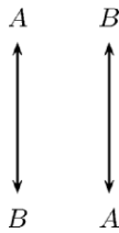
Fig. 2. Placement of test masses in a more advanced version of POEM. In the double difference observable, the EP violating signal adds and many errors cancel.
