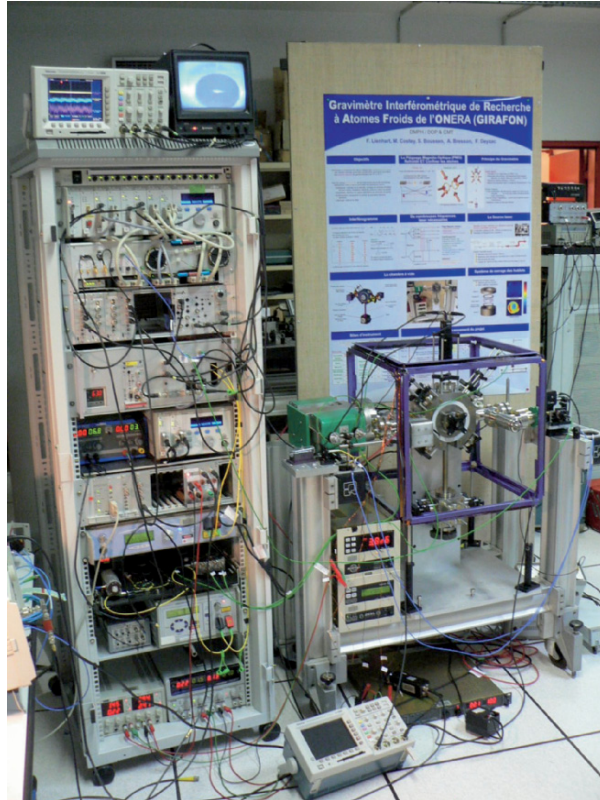
Fig. 6. The Girafon gravimeter which is being constructed at ONERA, Palaiseau.
