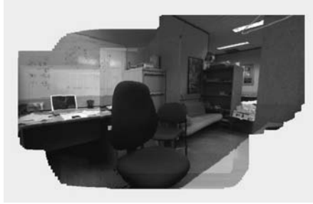
Fig. 2. Online output of the active rectification process: mosaic of rectified frames from right CeDAR camera.
