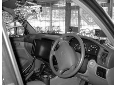
Fig. 4. Inside the ANU/NICTA intelligent vehicle. Cameras to monitor the road scene appear in place of the rear-vision mirror.
