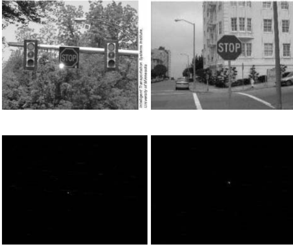
Fig. 5. Images of two stop signs from the internet, and corresponding regular polygon transform image using the algorithm presented for radius 20, and 28 respectively. Although not completely clear to eye in this reproduction, in both cases the sign is detected as the highest peak in the image.
