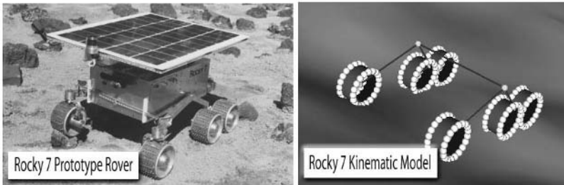
Fig. 3. Rocky 7 Prototype Mars Rover Kinematic Model: On the left is a picture of the Rocky 7 rover, a six-wheeled robot which has a rocker-bogie suspension to navigate complex terrain while maintaining wheel contact. On the right is a representation of our kinematic model of the suspension, which has the three passive joints (\rho, \beta_1, \beta_2) .
