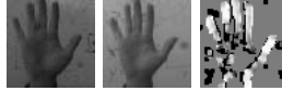
Fig. 4. NCC of 3x3 pixel regions at same coordinates in left and right images. Correlation results with higher values shown more white.
