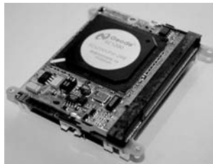
Fig. 5. The x-board based, 40 g and 56x71 mm computer module.
