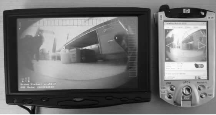
Fig. 2. Example LCD screen tested for lower arm mounting. The contrast is, however, a major challenge for outdoor usage. The screen is shown together with a corresponding iPAQ interface that can be used for portable control, but again with contrast issues
