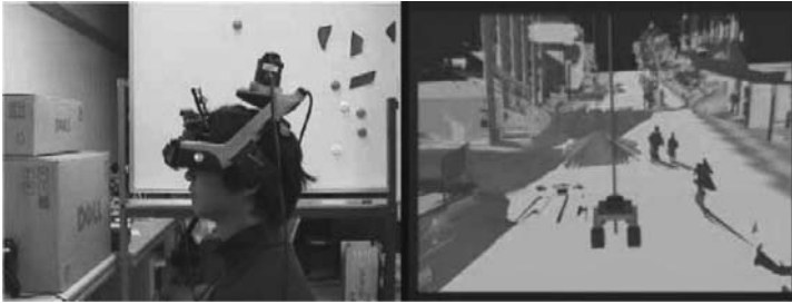
Fig. 10. A snap shot of the developed MR-based telepresence display (right) that is interactive with the operator’s head motion (left)
