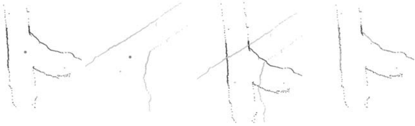
(a) 2D alignment: Each map is centered around its Voronoi node, and then one map is rotated relative to the other to find the minimum MSE alignment.
