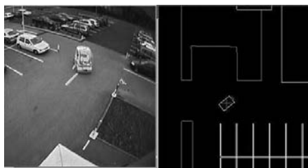
Fig. 4. The ParkView platform: left ) camera view of the Cycab experimental car moving in the parking lot of the laboratory; right ) the Cycab as detected on the tracking system.
