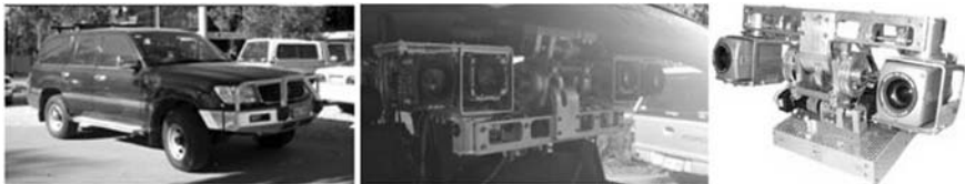
Fig. 1. Research platform. Left: Smart Car , and CeDAR mounted behind the windscreen (centre). Right: CeDAR, laboratory apparatus.
