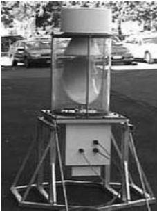
Fig. 5. Outdoor scanning terrain imaging millimeter-wave radar unit
