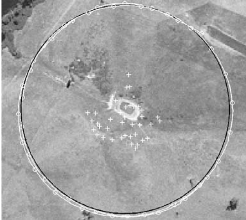
Fig. 11. An orbit around a feature (dam). The desired path (black line, 170 m radius) and navigation solution (white line) are indicated. At 1 second intervals, the position of the FV (white circles), and the projected centre of the sensor frame on the ground (white crosses) are shown.
