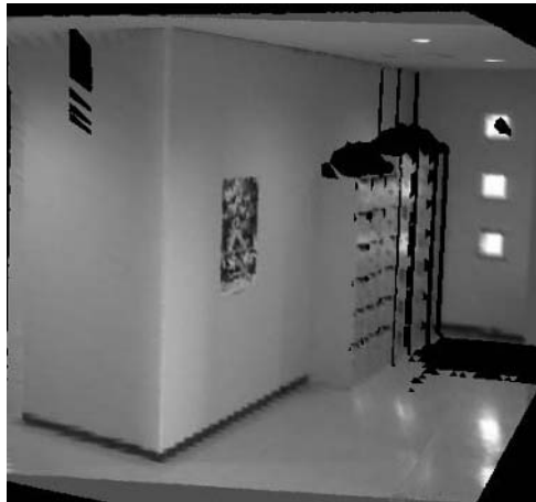
Fig. 9. A texture-mapped representation of the 3D geometry model
