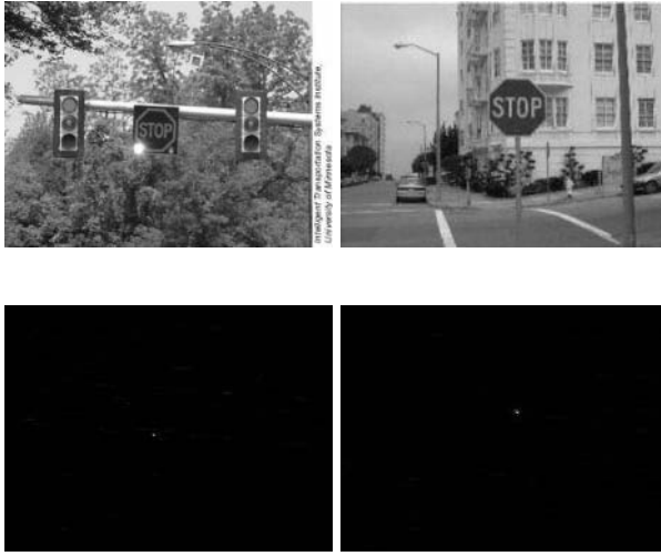
Fig. 5. Images of two stop signs from the internet, and corresponding regular polygon transform image using the algorithm presented for radius 20, and 28 respectively. Although not completely clear to eye in this reproduction, in both cases the sign is detected as the highest peak in the image.
