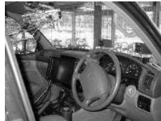
Fig. 5. Inside the ANU/NICTA intelligent vehicle. Cameras to monitor the road scene and find obstacles appear in place of the rear-vision mirror.
