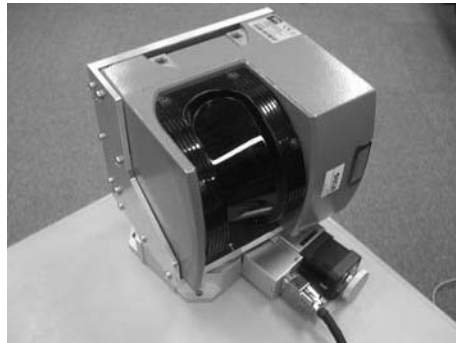
Fig. 6. A line laser scanner (SICK, LMS291) mounted on a turntable
