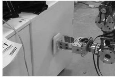
Fig. 15. Insertion with compliance motion
