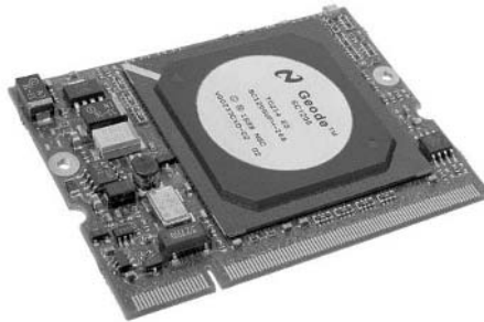
Fig. 3. X-board <861> single board computer from Kontron
