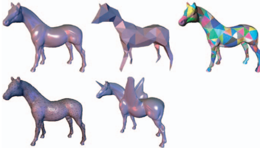
Fig. 5. Multiresolution adaptive parameterization of surfaces. Overview of the algorithm. Top left: a scanned input mesh (courtesy Cyberware). Next the parameter or base domain, obtained through mesh simplification. Top right: regions of the original mesh colored according to their assigned base domain triangle. Bottom left: adaptive remeshing with subdivision connectivity. Bottom middle: multiresolution edit. Figure reproduced from [47].
