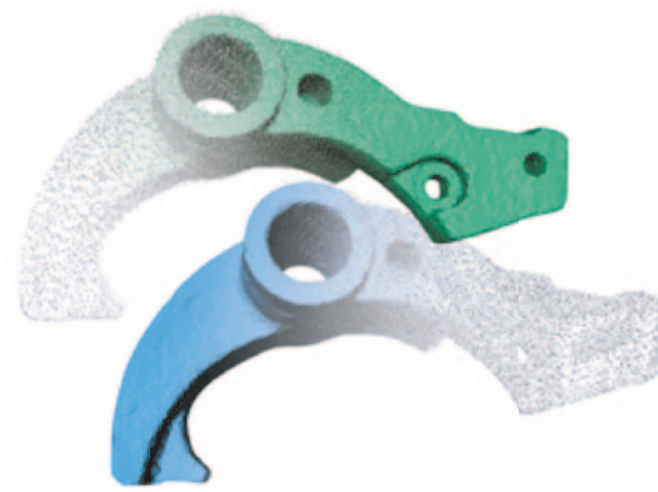
Fig. 6.28. Mechanical part, 12k points. Reconstructed with [56]
