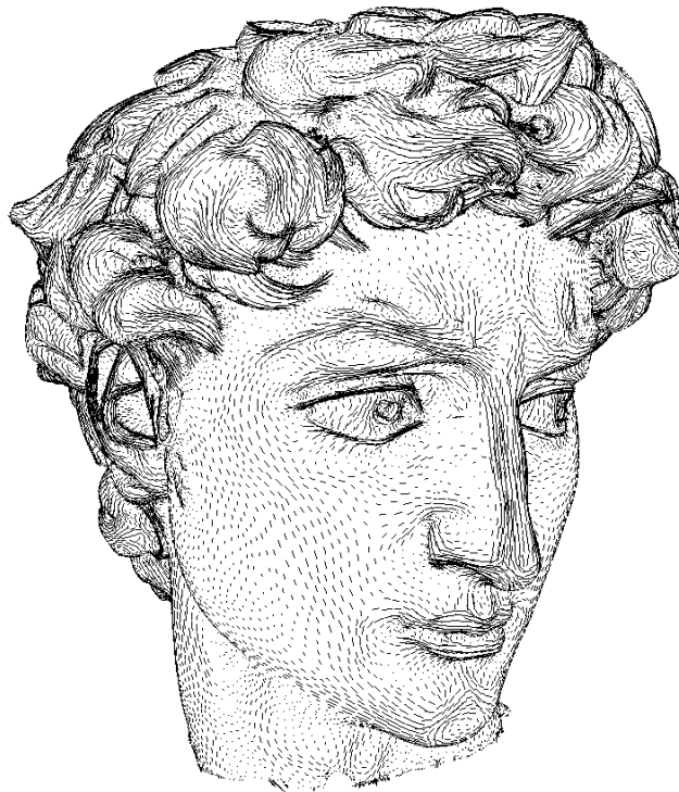
Fig. 4.7. Directions of minimal curvature estimated on a mesh of Michelangelo's David. For each vertex, the averaging domain used for computations is the 2-ring of that vertex
