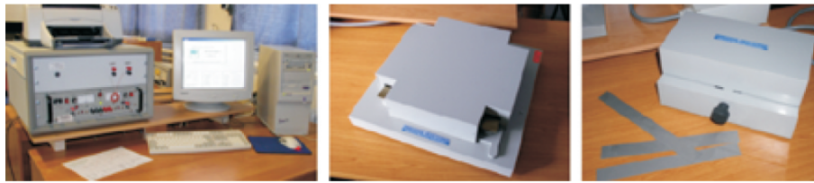
Fig. 6. REMACOMP Gauging system for magnetic characteristics measuring of constructional materials in dynamic fields 1Hz - 10 kHz. Epstein frame (in the middle). SST yoke (right)
