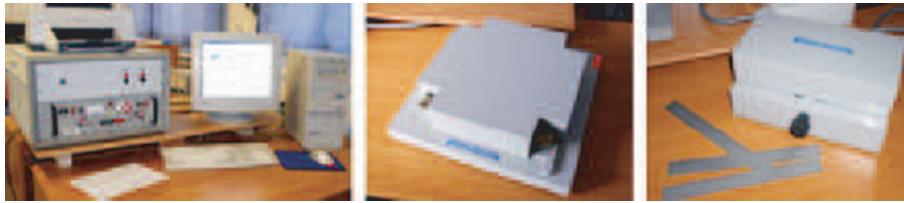
Fig. 6. (p. 238) REMACOMP Gauging system for magnetic characteristics measuring of constructional materials in dynamic fields 1Hz 10 kHz. Epstein frame (in the middle). SST yoke (right)
