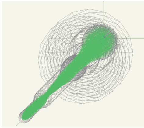
Fig. 4. 3-D plot of emitted electron trajectories
