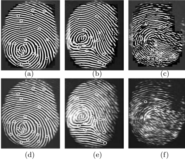
Fig. 4. Sensitivity to the tuning parameters of an enhancement algorithm. Input images are those shown in Figures 3(a-c). Panels (a-c) are obtained using E while panels (d-f) are obtained using E' . Minutiae consistently extracted from both algorithms are considered robust (o), whereas minutiae detected only by E or E' are non-robust ( \times )
