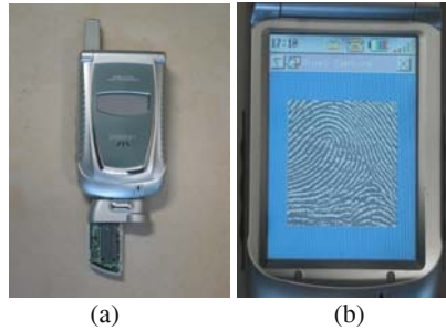
Fig. 5. (a) The appearance of the fingerprint recognition mobile phone; (b) Fingerprint image captured by the fingerprint recognition system
