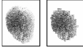
Fig. 2. Foreground/Background in the input fingerprint image: (a) Input fingerprint image, (b) Segmented image
