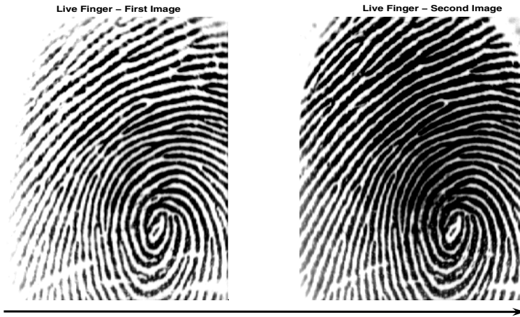
Fig. 1. The fingerprints captured as a time sequence. The left figure is captured at zeroth second, while the right is captured after five seconds. Perspiration is observed as time progresses in live fingers
