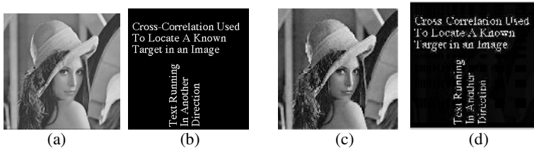
Fig. 3. Illustration of the robustness of ICA demixing ability with respect to JPEG compression. (a-b) the original images. (c-d) the extracted image from compressed mixtures of the originals
