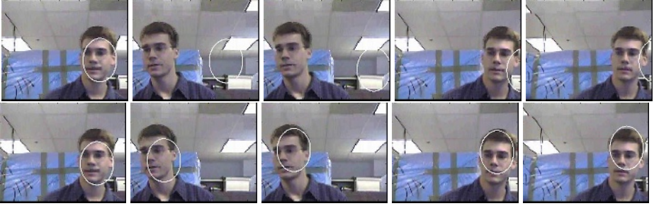
Fig. 5. Tracking results with the conventional PF (top) and the UAPF (bottom). From left to right, the frame numbers are 4, 7, 15, 30. At frame 7, the conventional PF tracker is trapped in a false region when the subject's face changes its motion direction suddenly. The conventional PF tracker fails for most the remaining frames and never be recovered
