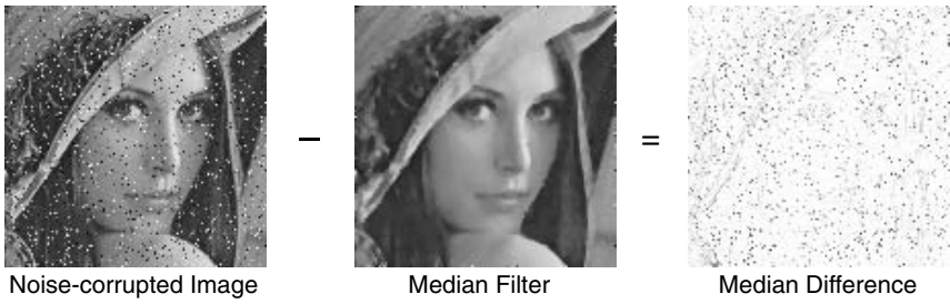
Fig. 3. Demonstration of median difference filter on “Lena”. For illustrative purposes the image contains 10% noise
