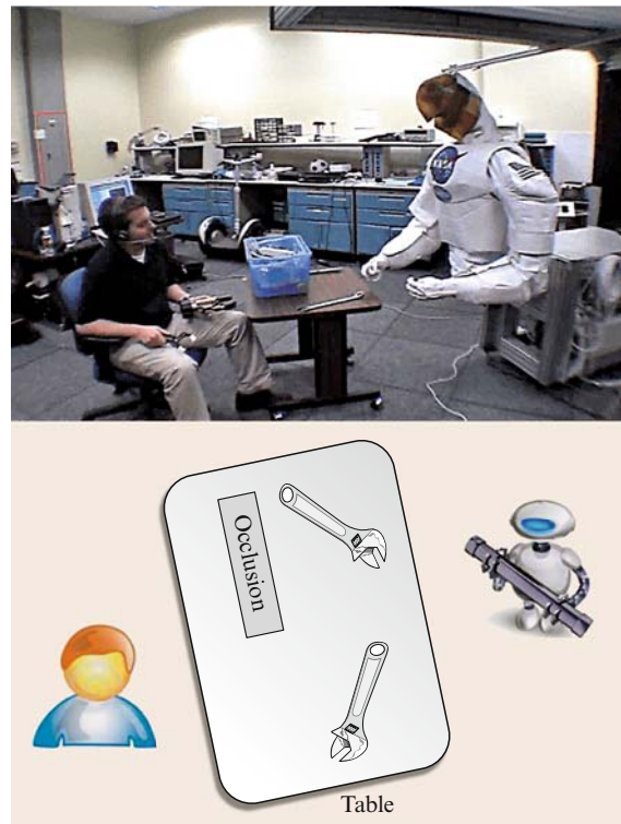
Fig. 58.13 Robonaut using visual perspective taking to disambiguate the intended referent when asked to hand me the wrench . The human can only see one wrench, but the robot can see both. The robot correctly hands the wrench that both can see
