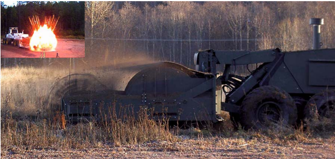
Fig. 48.5 Flail machine using hammers on the ends of spinning chains to clear vegetation and tripwires. This machine will also detonate a proportion of buried mines ( inset ) (photos Scanjack AB, Sweden)
