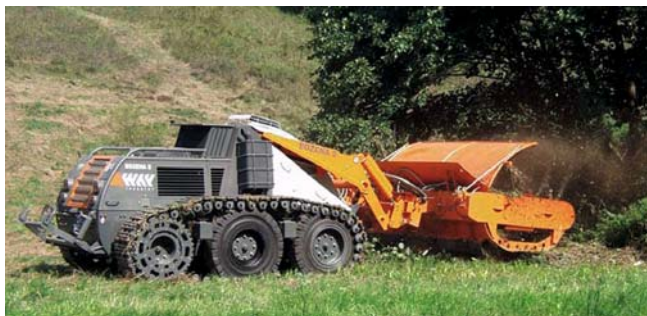
Fig. 48.7 Bozena teleoperated demining vehicle (Way Industry, Slovakia)
