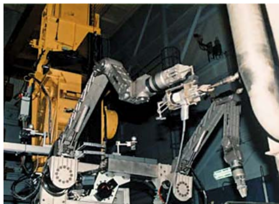
Fig. 48.15 Dual-arm D&D manipulator system (courtesy of Oak Ridge National Laboratory)
