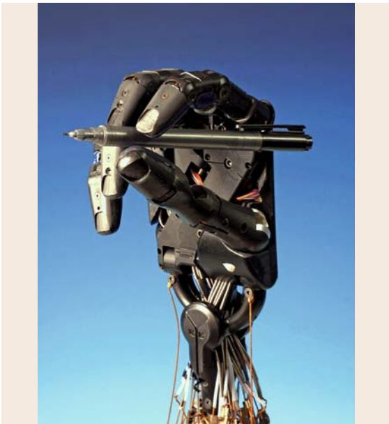
Fig. 28.6 This grasp has a force closure grasp appropriate for dexterous manipulation (Image of Shadow Dextrous Hand © Shadow Robot Company 2008)
