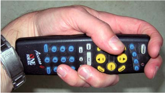
Fig. 28.5 The palm, fingers, wrist, and watch band combine to create a very secure form closure grasp of a TV remote controller
