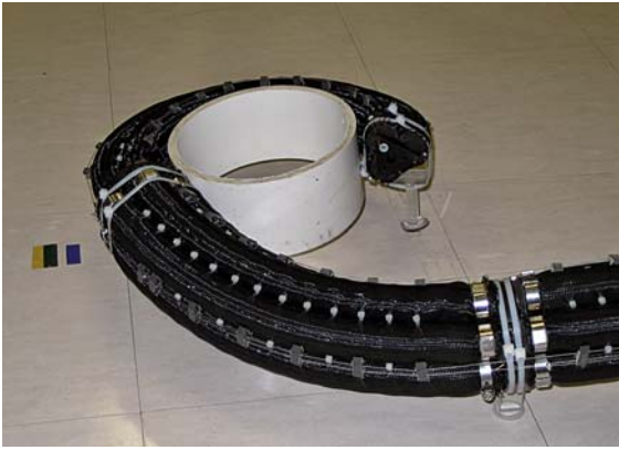
Fig. 11.7 The OctArm continuum manipulator (courtesy I. Walker)
