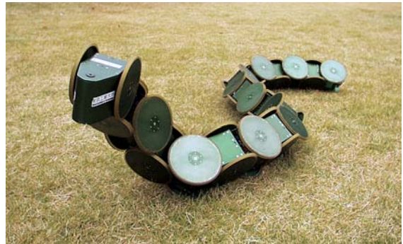
Fig. 11.6 Active cord mechanism (courtesy S. Hirose)
