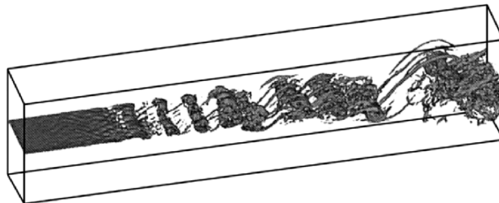
Fig. 10.15. A global view of the vortical structures in a mixing layer. From Lesieur et al. (2000)
