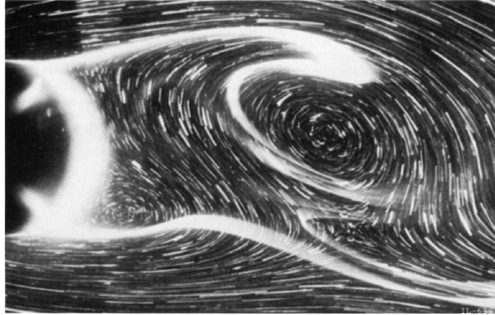
Fig. 2.2. Streamlines and streaklines in unsteady vortex shedding from a circular cylinder. From Taneda (1985)
