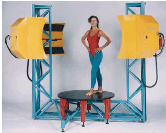
Fig. 16.1. 3D body scanner
