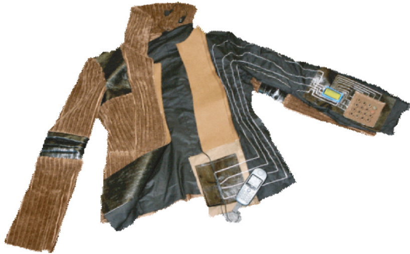
Fig. 6.12. Communication jacket with embroidered conductor lines
