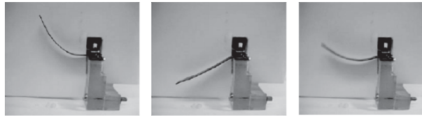
Fig. 4.22. A 200 \mu\text{m} thick IPMC strip that shows significant bending due to a 2 V potential
