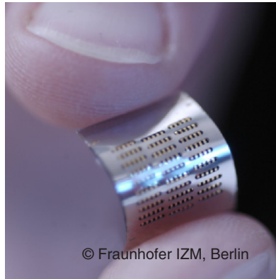
Fig. 5.30. Flexible micro-fuel cell demonstrator: size 1\text{ cm}^2 , thickness 200\text{ }\mu\text{m} , 80\text{ mW cm}^{-2}
