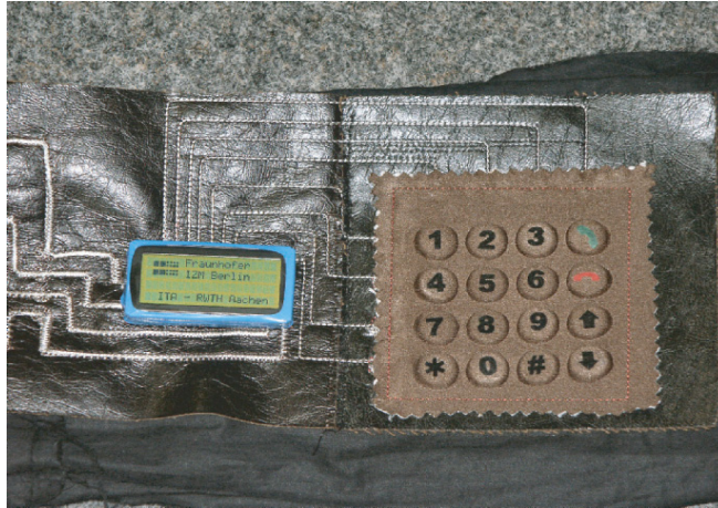
Fig. 6.13. Detail of embroidered circuits in sleeve
