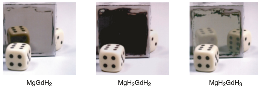
Fig. 4.6. Reversible hydrogen uptake by a thin Pd-coated \text{MgGdH}_2 film with associated optical changes
