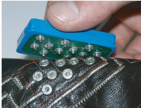
Fig. 6.8. Detachable interconnection by snaps for a display module
