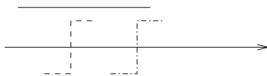
Fig. 3 The dot product between a wavelet and a histogram is zero unless the support of the wavelet intersects a boundary of the histogram
