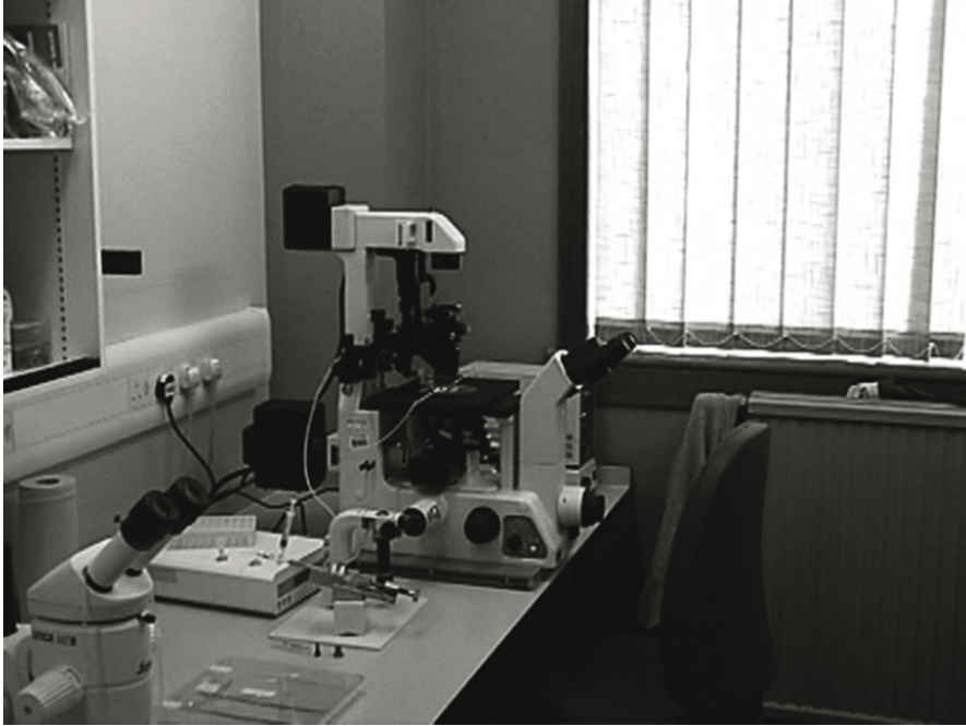
Fig. 8.1. Nikon inverted microscope fitted with Narishige micromanipulators and microinjectors
