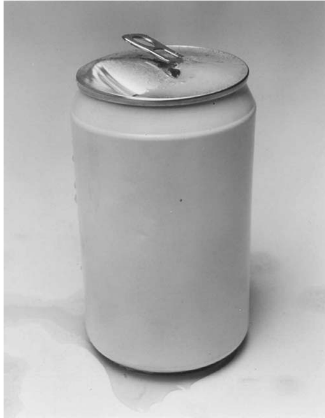
Fig. 11.1. “Blown” packages of food or beverages represent the most obvious sign of yeast spoilage. This soft drink was inoculated with Zygosaccharomyces bailii before capping. Similar cans of beverage distended, ruptured or exploded between 1 month and 2 years
